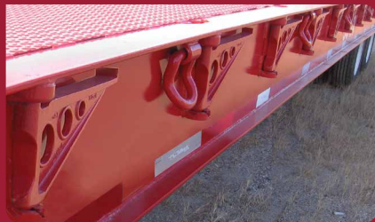
Steel I-beam crossmembers on 9 in. centers provide the framework for the rugged Talbert TA Series.
