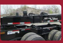
70" Gooseneck Extension and convertible Jeep Dolly with removable axles, sliding 5th wheel, and multiple kingpin settings.
