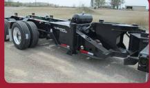
E2Nitro™ distributes weight to rear axle group via hydraulic / nitrogen accumulator system; dampening axle movement and controlling load transfer.
