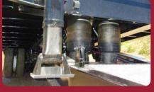
Pneumatically operated tilting deck and ramp design.
