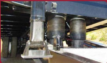
Pneumatically operated tilting deck and ramp design.
