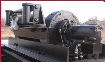
Heavy-duty planetary winch, standard with Talbert, is operated by a wireless remote control, delivering maximum pulling power.
