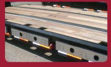
Ultra-low deck height for unmatched Multiple gooseneck options clearance and simplified route logistics. (pictured with optional aluminum pullouts)
