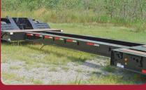
Increased camber as deck opens due to extensive deck length, offering greater hauling capabilities.
