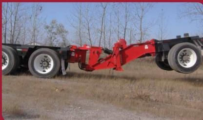
The E1Nitro™ is designed for trailers with up to 60-ton capacities and can carry 24,700 pounds in its 3+1 configuration.
