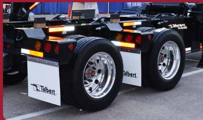
The E2Nitro™ is designed for trailers with up to 70-ton capacities and can carry 49,400 pounds in its 3+2 formation.
