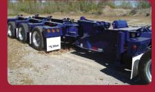
The E3Nitro™ is designed for trailers with up to 85-ton capacities and can carry 74,100 pounds in its 3+3 configuration.
