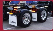
The E2Nitro™ is designed for trailers with up to 70-ton capacities and can carry 49,400 pounds in its 3+2 formation.
