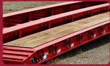
Rugged, fabricated T-1 steel side rail providing industry-leading low 15-1/2 in. loaded deck height in track area.
