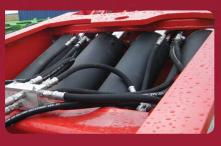
Robust, low-pressure, four-cylinder hydraulic removable gooseneck maximizes lift capacity and load height.
