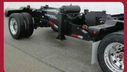
Allows users to operate as a 3+1 spread-axle with the E1Nitro™. Can also function as four axle close coupled.
