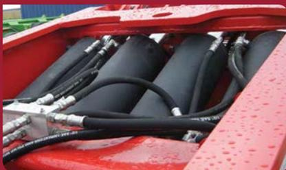
Robust, low-pressure, four-cylinder hydraulic removable gooseneck maximizes lift capacity and load height.
