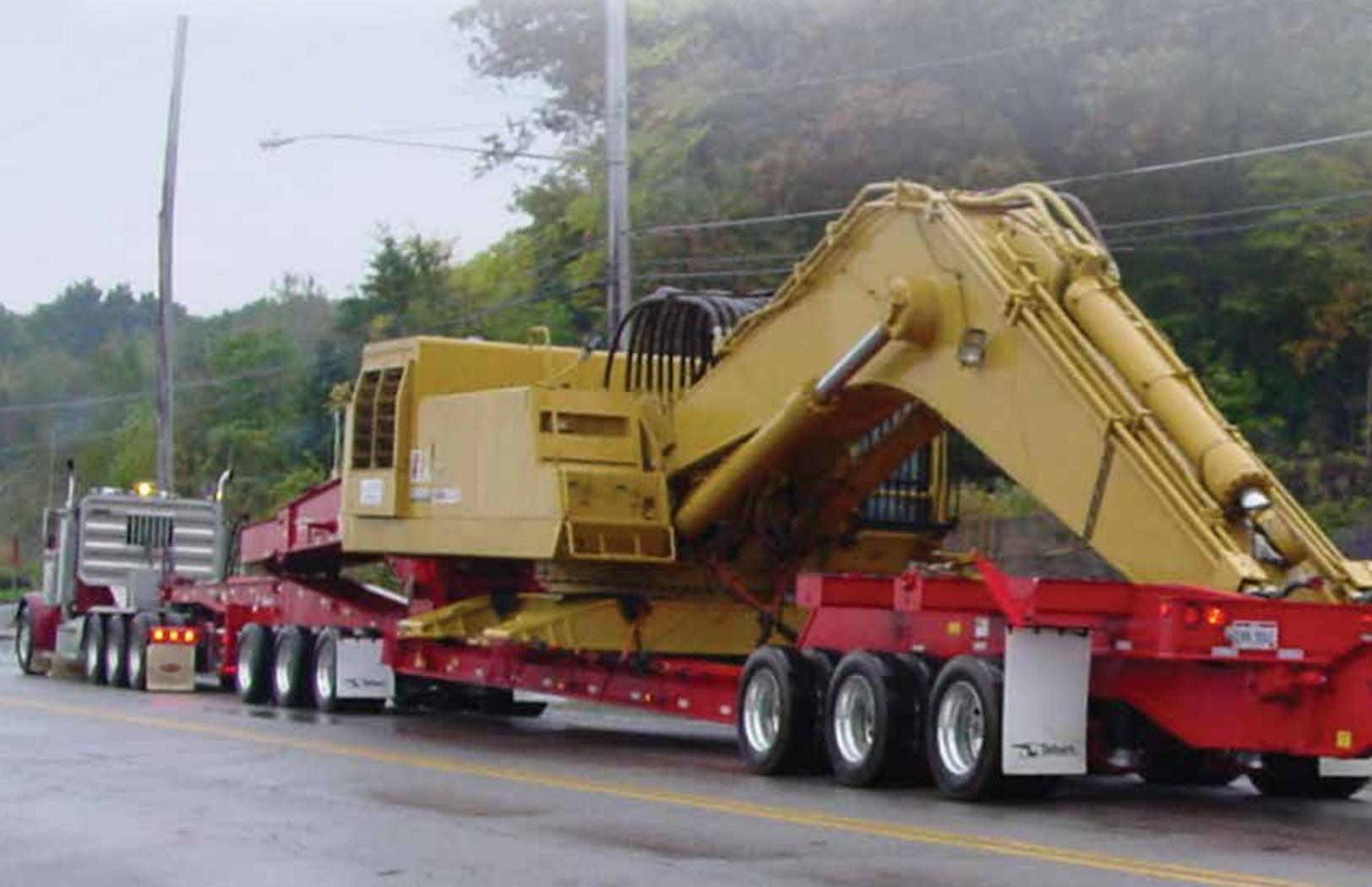
80 Ton, 13 Axle, Inboard West Coast Suspension
