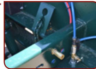
Chain Lift with Air Bag Isolation Valve
