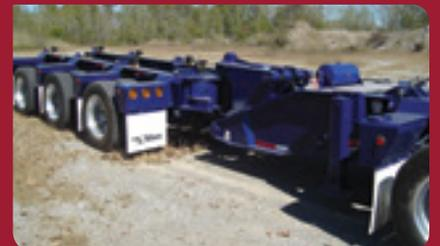
The E3Nitro™ is designed for trailers with up to 85-ton capacities and can carry 74,100 pounds in its 3+3 configuration.
