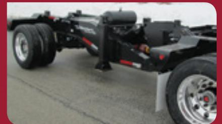
Allows users to operate as a 3+1 spread-axle with the E1Nitro™. Can also function as four axle close coupled.
