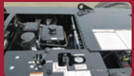
E2Nitro™ is standard with gas engine power pack to drive loading cylinders via controls shown.
