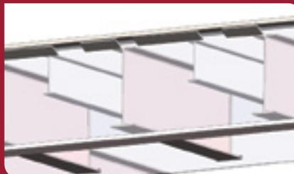
Rugged, heavy-duty deck courtesy of auxiliary cross-members and top flange reinforcement.
