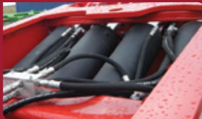
Robust, four-cylinder hydraulic removable gooseneck maximizes lift capacity and load height.
