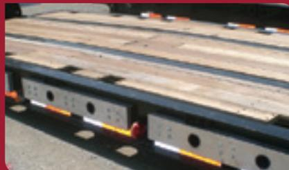
Ultra-low deck height for unmatched clearance and simplified route logistics. (pictured with optional aluminum pullouts)
