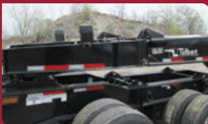
70" Gooseneck Extension and convertible Jeep Dolly with removable axles, sliding 5th wheel, and multiple kingpin settings.
