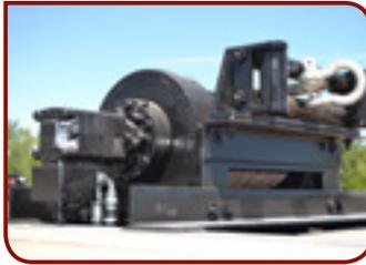
20,000# Planetary Winch w/ Air Tensioner & Cable Roller Guide
