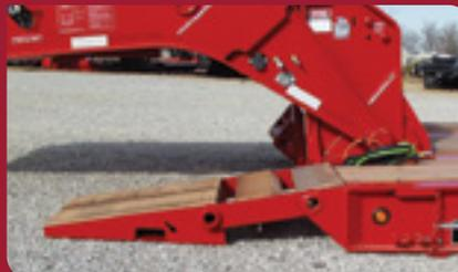
50" loading ramps are wood-filled and double-hinged, providing the strength and traction needed for heavy track equipment.
