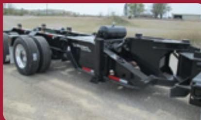
E2Nitro™ distributes weight to rear axle group via hydraulic / nitrogen accumulator system; dampening axle movement and controlling load transfer.
