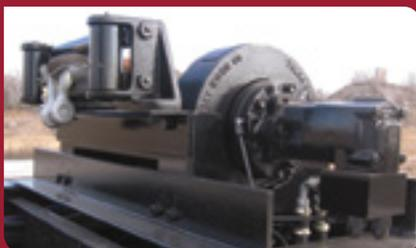
Heavy-duty planetary winch, standard with Talbert, is operated by a wireless remote control, delivering maximum pulling power.
