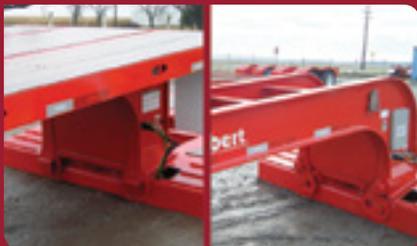
Sliding pin or swinging teardrop connections available for enhanced tractor compatibility.
