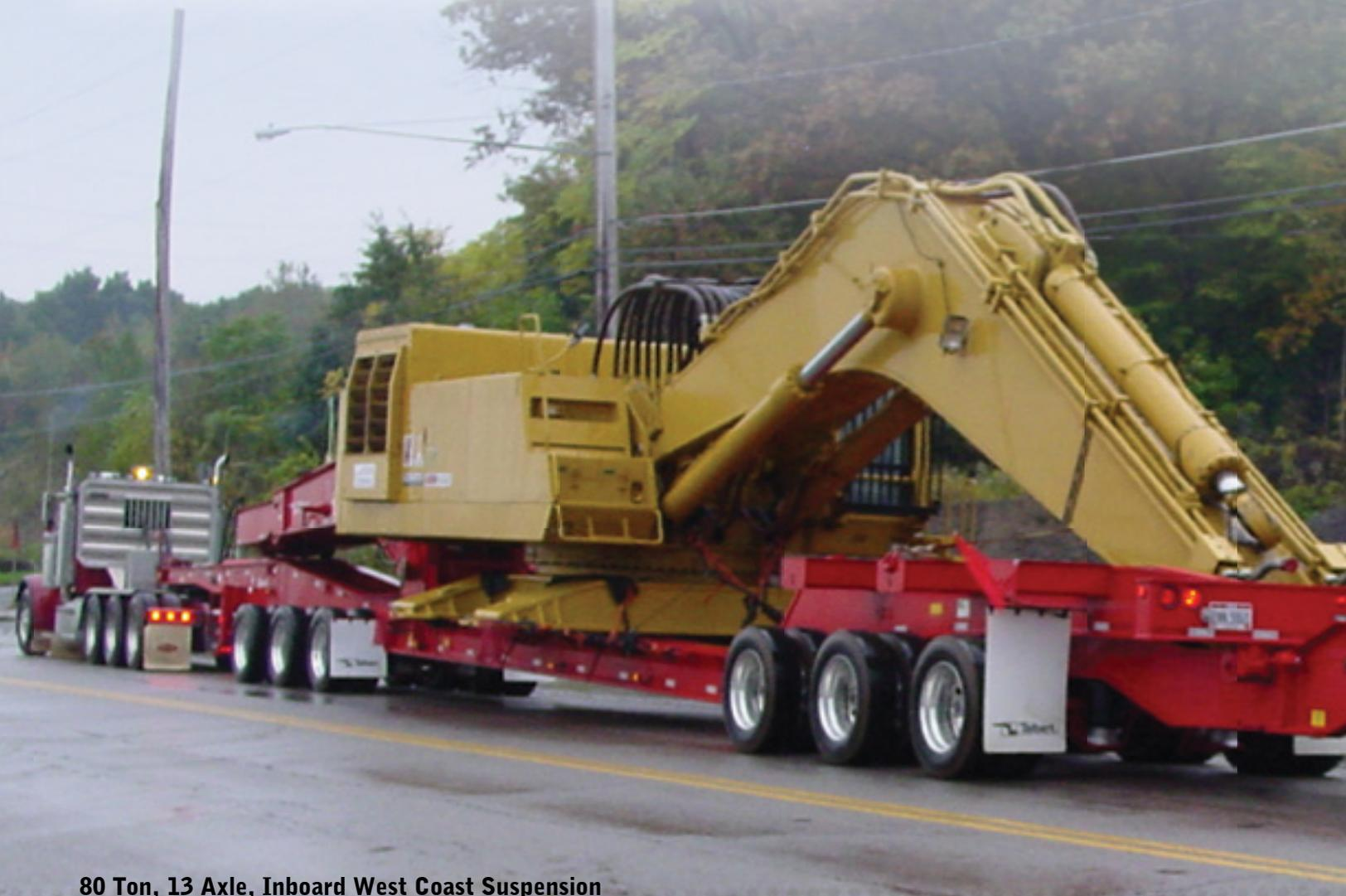
80 Ton, 13 Axle, Inboard West Coast Suspension
