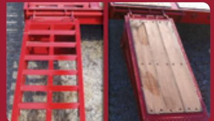
Self-cleaning or optional wood-filled ramps; choose the ramp that's right for your load!
