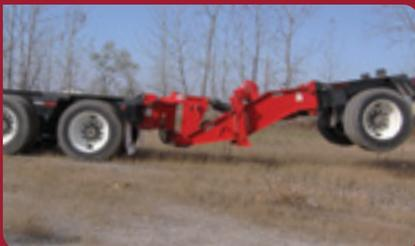
The E1Nitro™ is designed for trailers with up to 60-ton capacities and can carry 24,700 pounds in its 3+1 configuration.
