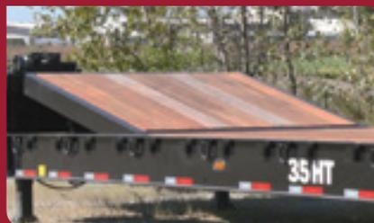
The hydraulic front ramp offers a convenient method for gooseneck loading.
