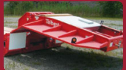
Optional steel gooseneck fenders with clearance lights protect the tractor and the load from road spray.
