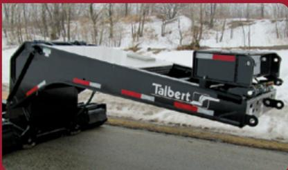
Optional 24 in. flip gooseneck extension (increasing swing radius to 132 in.) allows greater load transfer capability.
