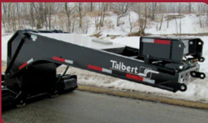
Optional 24 in. flip gooseneck extension (increasing swing radius to 132 in.) allows greater load transfer capability.
