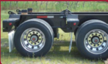
3rd axle and 4th axle attachments can be used as 3 or 4-axle close couple, 3+1 or 2+2 spread axle.
