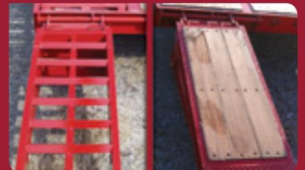
**Self-cleaning or optional wood-filled ramps; choose the ramp that's right for your load!**
